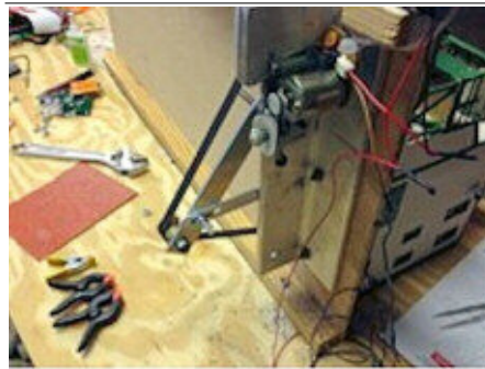
The improved drive mechanism features a new drive pulley and idler arm.
